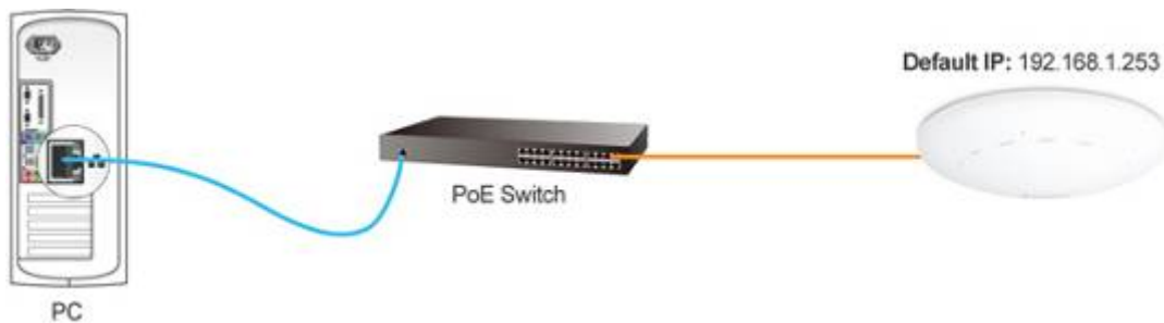
Figure 5-4 LAN Interface Setup Topology
