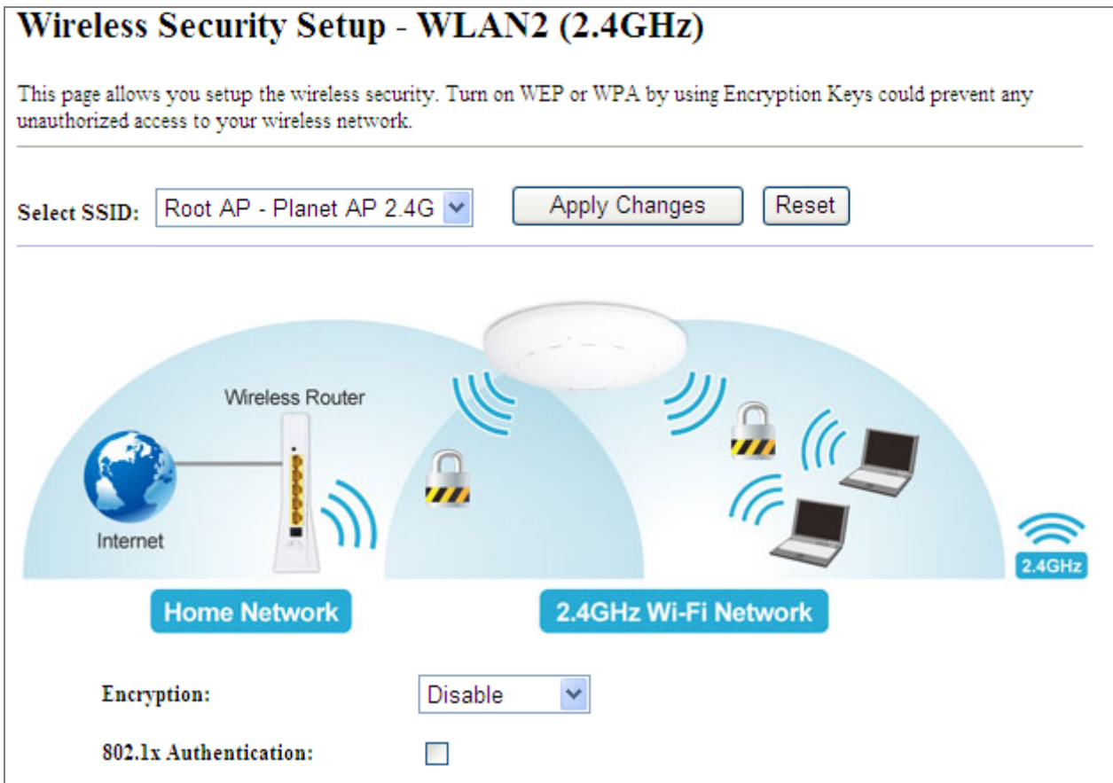
Figure 5-67 Wireless Security Settings – 2.4GHz
