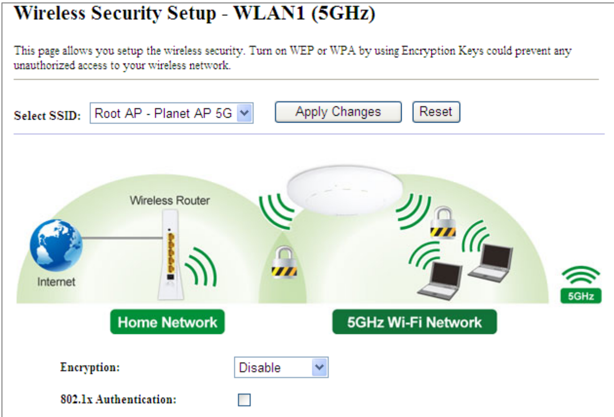
Figure 5-36 Wireless Security Settings – 5GHz
